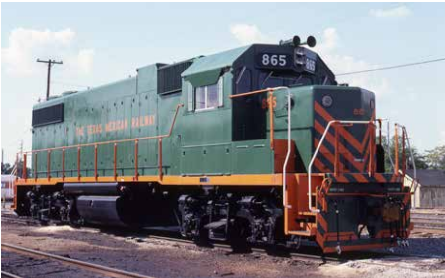
Texas-Mexican GP38 865 lacks dynamic brakes and snowplow, a nod to the terrain and climate of South Texas. It also placed two single-unit orders for the GP60. Michael A. Wise, Brian M. Schmidt collection
